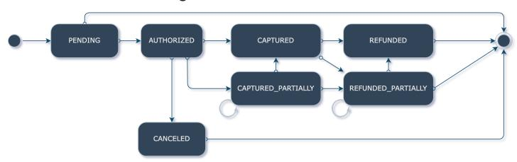
The transaction state diagram maps out the state flow on transactions.
